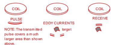
When the transmitted pulse hits a metal object, an electro-magnetic field is induced in the object. This causes eddy currents to flow in the metal, which in turn generates a second electro-magnetic field. This field is picked up by the coil, amplified and then displayed by the meter and heard in the earphones.
