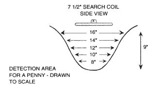
The above illustration represents the detection area for a penny, a larger object would have a larger detection area. Due to the large detection area of the PULSE 8X, a variable sensitivity switch is provided. This enables the sensitivity to be decreased, once a target is detected, to allow easy pinpointing of the target.
