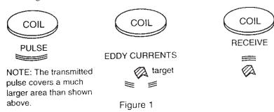
When a transmitted pulse hits a metal object, a magnetic field is induced in the object. This causes eddy currents to flow in the metal, which in turn generates a second magnetic field. This field is picked up by the coil, amplified, and then displayed by the meter and heard in the speaker/earphone.
